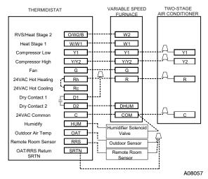
Edge Thermidistat Models TP-PRH-01 & TP-NRH-01 w/ Furnace & 2-Stage Air Conditioner
